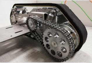
In order to be able to climb vertically the extremely slippery surfaces the robot has been designed as a tracked vehicle, equipped with two robust rubber belts which are keep in contact with the surface thanks to a powerful vacuum-based adhesion system, placed at the center of it. The two aforementioned rubber tracks allow the robot to move on the metal surfaces with two different degrees of freedom; it can goes back/forth and rotate, even on its main axis.
