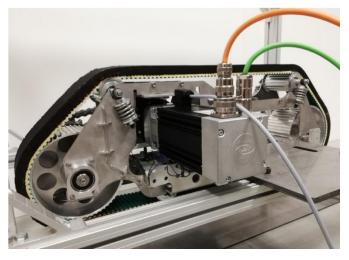
In order to be able to climb vertically extremely slippery surfaces, the robot has been designed as a tracked vehicle, equipped with two robust rubber belts, which keep contact with the surface, thanks to a powerful vacuum-based adhesion system, placed at the its centre. The two aforementioned rubber tracks allow the robot to move on the metal surfaces with two different degrees of freedom; it goes back/forth and rotates, even on its main axis.
